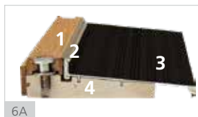
Cross section of aluminum inswinging sill 1. Wood species of sill matches door 2. Adjustable hardwood sill cover 3. Durable anodized sill coating 4. Composite subsill
