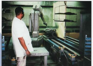
Components to be painted by this robot are placed in a holding fixture and covered by a custom mechanical mask. The automated shuttle then transports the fixture into the booth where the robotically controlled paint gun sprays the exposed area.
