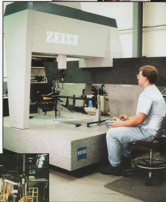
This Zeiss Coordinate Measuring Machine (CMM) provides accurate dimensional analysis for complete geometric inspections. This CMM has a measuring envelope of 46" (x-axis) x 78" (y-axis) x 24" (z-axis).
