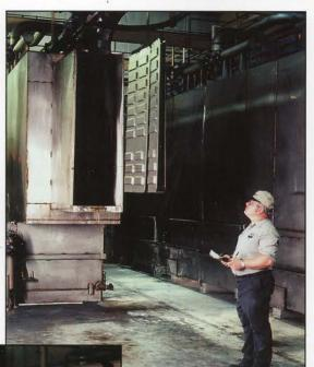
An eight stage pretreatment process consisting of an alkaline cleaner, multiple water rinses, an iron phosphate conversion coating, a nonchrome acid seal rinse, a deionized water rinse and a drying and preheating oven prepare the surfaces for powder coating. Lab technicians titrate the pretreatment tanks and monitor fluid levels and temperatures every four hours for consistent cleaning and coating results.
